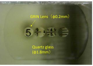
4-chnnel Integrated GRIN lens (outer-diameter: φ1.8mm, lens diameter:200microns, lens pitch:250 microns )
