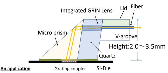
Straight-type Low Profile Couplers for Silicon Photonic dies
